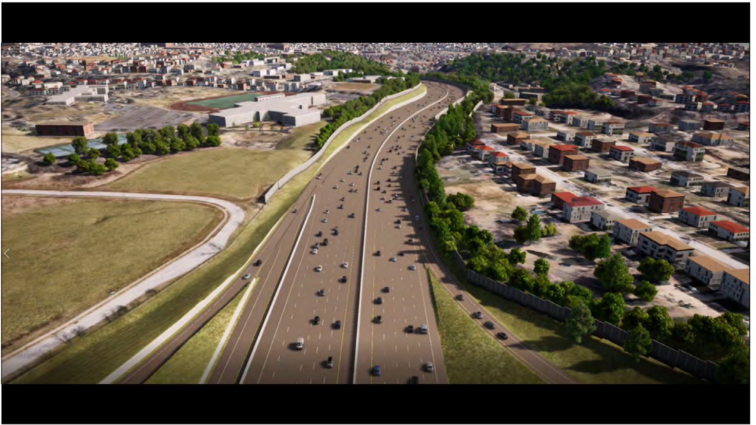
This slide shows what the finished project might look like from Kyles Lane. Notice the noise wall system in Fort Wright along the east side of the highway. On the west side, notice the noise wall constructed at the top of the slope adjacent to Notre Dame Academy.
