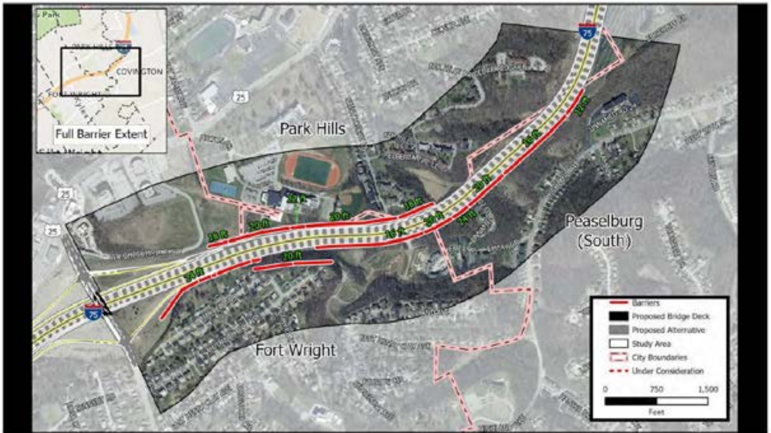
The red lines on this slide show noise walls that were evaluated as part of the noise study for Fort Wright. The green numbers show the heights of the different sections of the noise walls.
