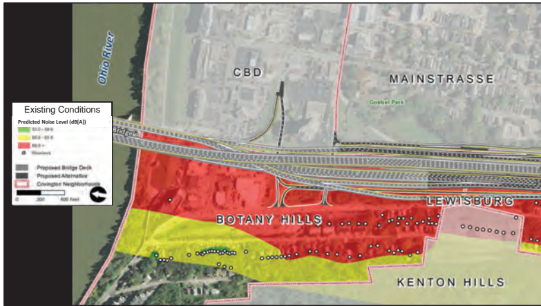
This slide highlights the receptors evaluated as part of the noise analysis. The color gradient indicates existing noise readings, with red representing areas with higher sound levels and green representing quieter areas.
