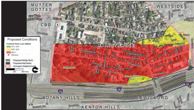
This slide shows how sound conditions are projected to change for the evaluated receptors by the year 2050 after the project is built. The color gradient indicates predicted noise levels, with red representing areas with higher sound levels and yellow representing moderate sound levels.
