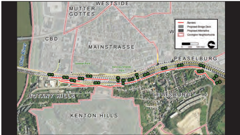
The red lines on this slide show noise walls that were evaluated as part of the noise study for northern Lewisburg and Botany Hills. The green numbers show the heights of the different sections of the noise walls.
