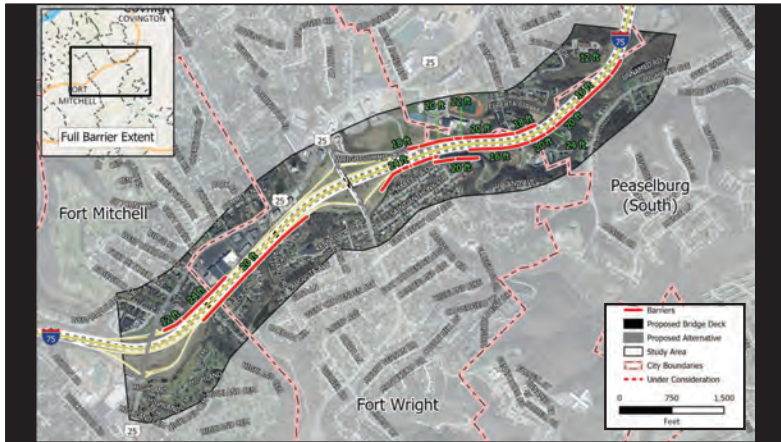
The red lines on this slide show noise walls that were evaluated as part of the noise study for Fort Wright. The green numbers show the heights of the different sections of the noise walls.
