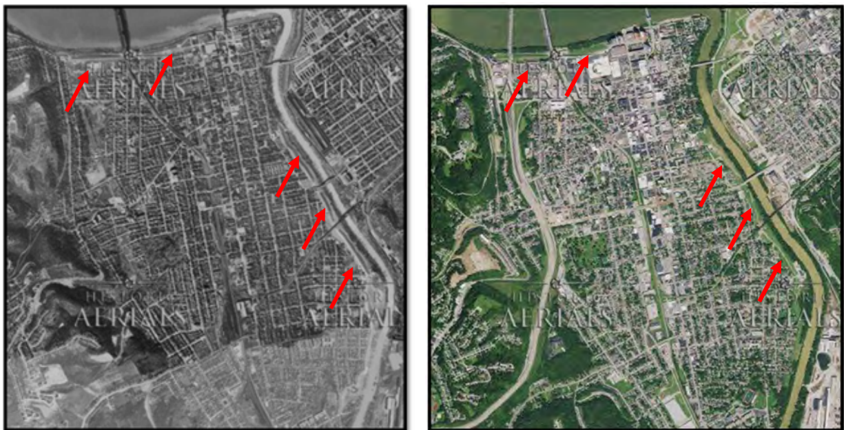
Figure 48. Covington Levee System. Aerial comparison showing the levee system has not experienced any significant changes from its original 1950s design. Left: 1955 aerial of Covington's Levee System. 201 Right: 2019 aerial of Covington's Levee System. 202 Note red arrows indicating earthen levee wall locations.
