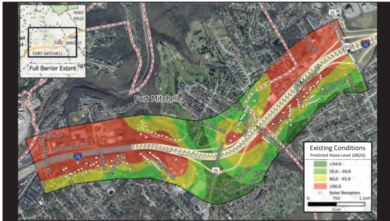
This slide highlights the receptors evaluated as part of the noise analysis for Fort Mitchell. The color gradient indicates existing noise readings, with red representing areas with higher sound levels and green representing quieter areas.
