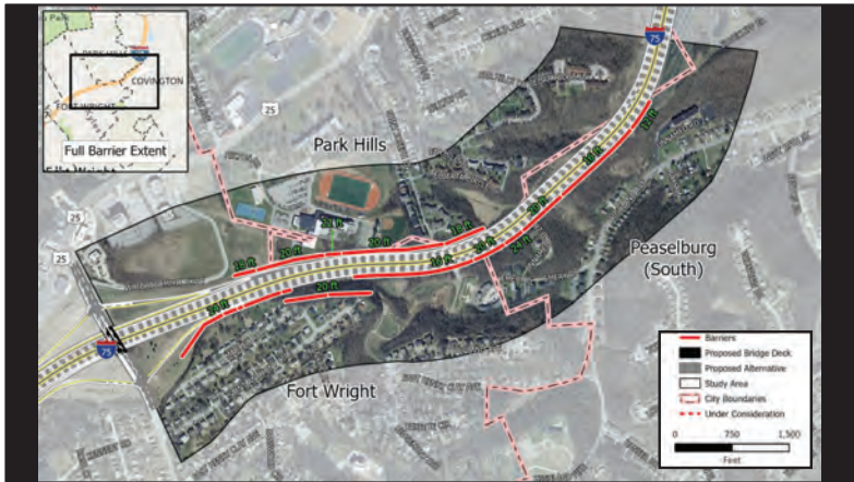
The red lines on this slide show noise walls that were evaluated as part of the noise study for Park Hills. The green numbers show the heights of the different sections of the noise walls.
