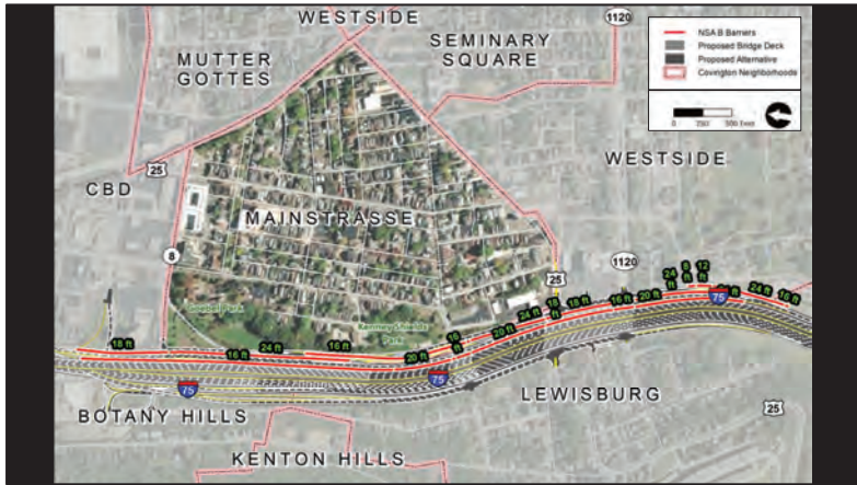
The red lines on this slide show noise walls that were evaluated as part of the noise study for Mainstrasse. The green numbers show the heights of the different sections of the noise walls.
