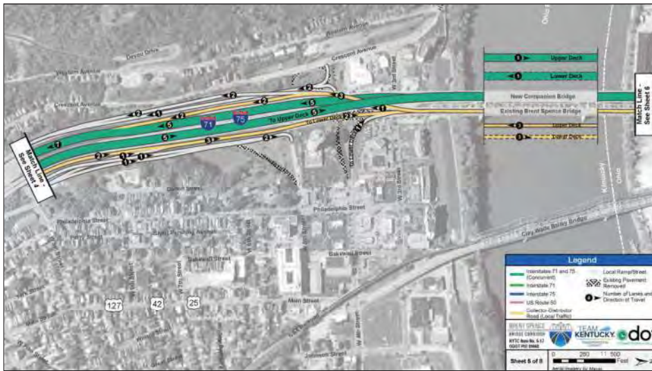
This slide shows how traffic will move across the Ohio River. Interstate traffic (shown in green) will use the companion bridge and stay on the interstate corridor to travel through Covington and Cincinnati. Local traffic will use ramps and the collector-distributor system to travel to destinations in Cincinnati and Covington.
