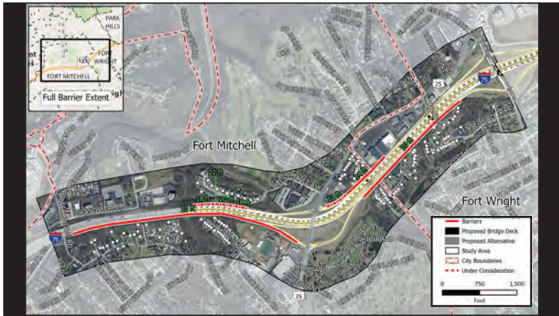
The red lines on this slide show noise walls that were evaluated as part of the noise study Fort Mitchell. The green numbers show the heights of the different sections of the noise walls.
