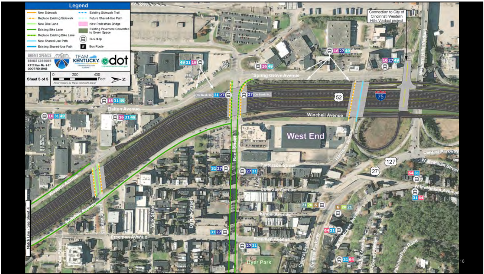
This exhibit shows some of the planned pedestrian and bicycle facilities near Camp Washington. Note the new shared use path on Harrison Avenue, the new bike lanes on Findlay Street, and the replaced sidewalks on Harrison, Bank, and Findlay. These will tie into the existing bike lanes on Western, Winchell, and Bank and connect to existing transit stops.
