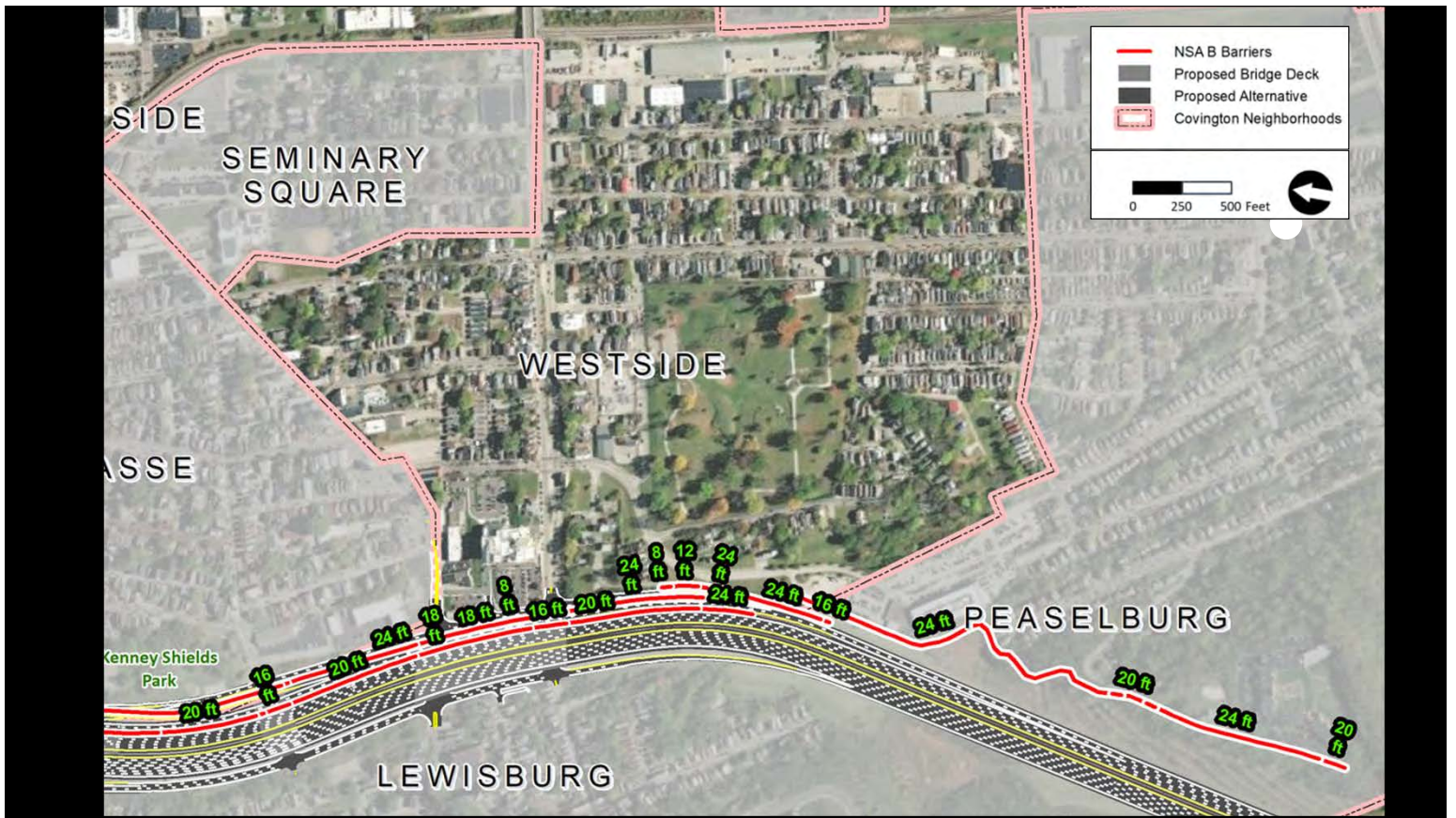
The red lines on this slide show noise walls that were evaluated as part of the noise study for in the Westside Covington area. The green numbers show the heights of the different sections of the noise walls.
