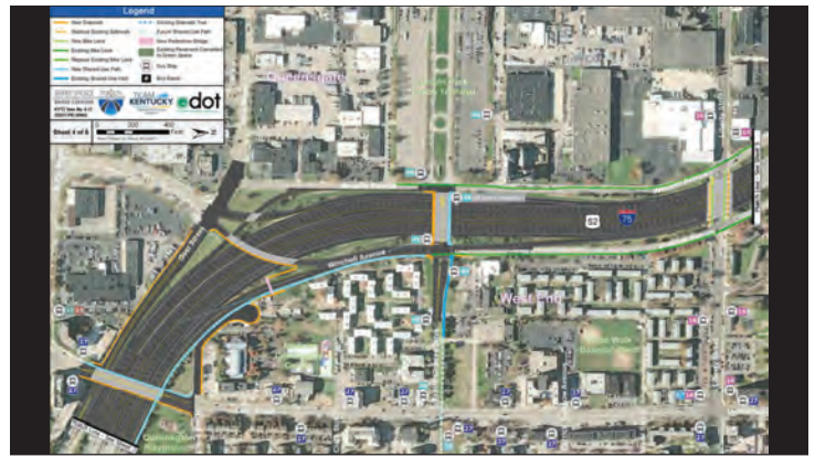
Continuing north, we see how the new shared use path on Winchell Avenue continues all the way to Ezzard Charles Drive. Also notice new shared use paths on Linn Street and Ezzard Charles Drive, new sidewalks along Guest Street, Court Street, Freeman, and Ezzard Charles, a new pedestrian bridge connection over Winchell Avenue, and new bike lanes on Liberty Street.
