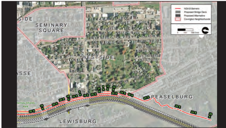
The red lines on this slide show noise walls that were evaluated as part of the noise study for in the Westside Covington area. The green numbers show the heights of the different sections of the noise walls.
