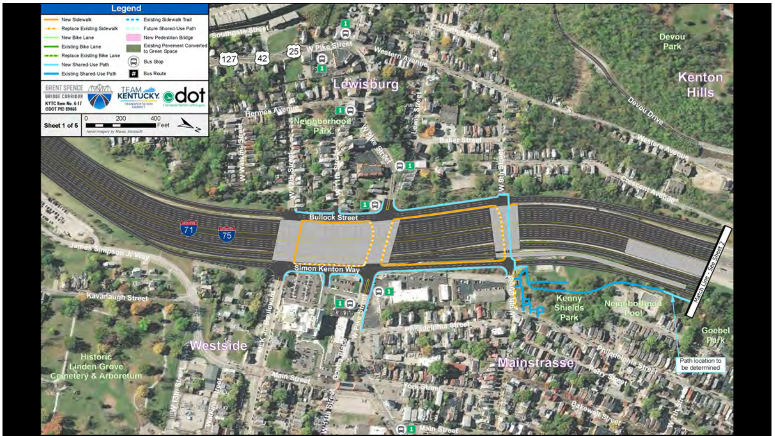
This exhibit shows some of the planned pedestrian and bicycle facilities near Peasenburg. Note the new shared use paths and sidewalks along the frontage roads. Also notice the new and rebuilt sidewalks under the MLK/West 12th, Pike, and West 9th Street bridges. A new shared use path will be built under the West 9th Street bridge, which will tie into the shared use paths in Goebel Park.
