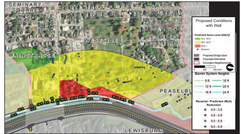
This slide shows predicted noise levels for the evaluated receptors under proposed (2050) conditions with construction of a noise wall. For the receptors, anything with light pink and dark pink have a reduction of 5 decibels and are considered benefitted receptors.
