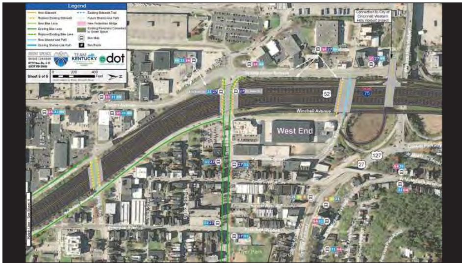
As we move further north, notice the new bike lanes on Findlay Street, the new shared use path on Harrison Avenue, and the replaced sidewalks on Harrison, Bank, and Findlay. These will tie into the existing bike lanes on Western, Winchell, and Bank. Throughout the corridor the new and improved pedestrian and bicycle facilities will provide connections to existing transit stops.
