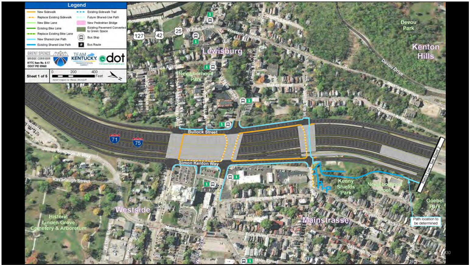
This exhibit shows some of the planned pedestrian and bicycle facilities near Mutter Gottes and the CBD. Note the new shared use paths and sidewalks along the frontage roads. Also notice the new and rebuilt sidewalks under the MLK/West 12th, Pike, and West 9th Street bridges. A new shared use path will be built under the West 9th Street bridge, which will tie into the shared use paths in Goebel Park.
